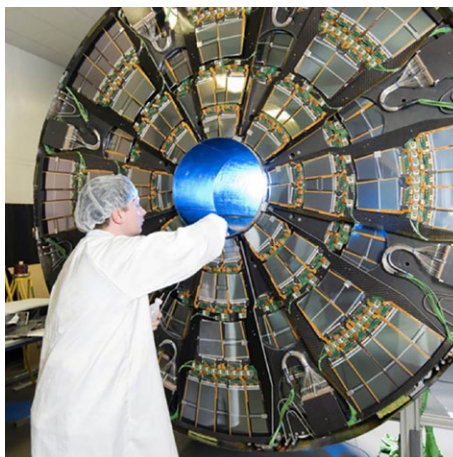
One end-cap of the CMS tracker is opened during installation work (Photo: CERN).
