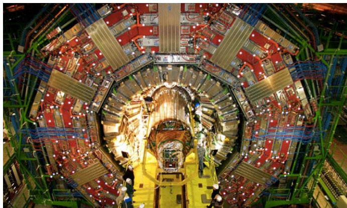
Installation of the world’s largest silicon tracking detector in the CMS experiment (Photo: CERN).
