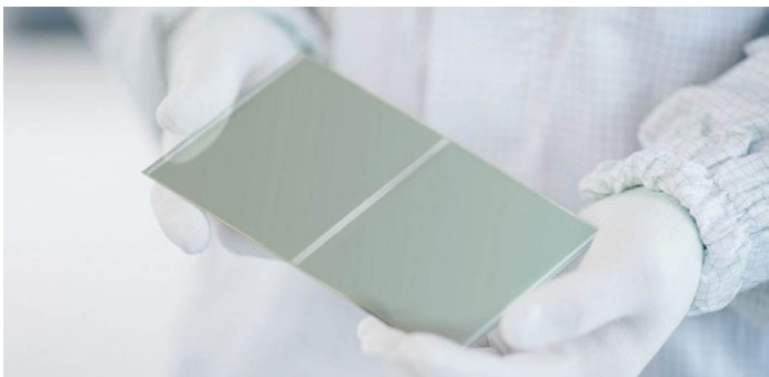
Elementary particle strip sensor released from the wafer (Photo: Infineon Technologies Austria AG).
